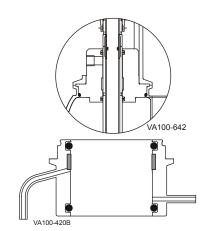
Figure 8 - External Steam Barrier - upper stem
