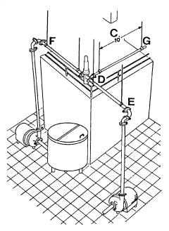
Figure 2 - Pipeline Support
