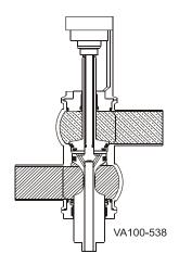
Figure 14 - Valve Closed
