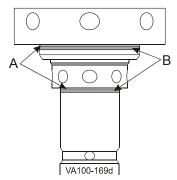
Figure 19 - Bottom edges align with scribe lines
