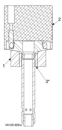
Figure 30 - Upper Stem Tef Flow® P Seat Removal (Kit # 132990+)
