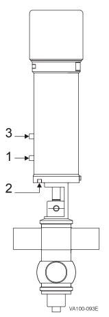
Figure 11 - Solenoid Valve Port Connections
