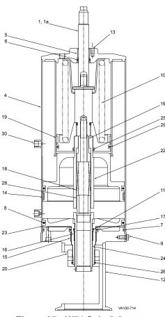
Figure 37 - W71 Sch. 5 Actuator Assembly (Seat Lift Valve)
