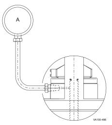
Figure 7 - Connection of Flush Supply
