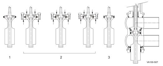
Figure 28 - Radial Seal Installation
